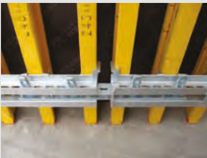
The strong wedge design provides necessary tension through the slotted waler connectors for leak-proof joints, while simultaneously aligning the panels.
