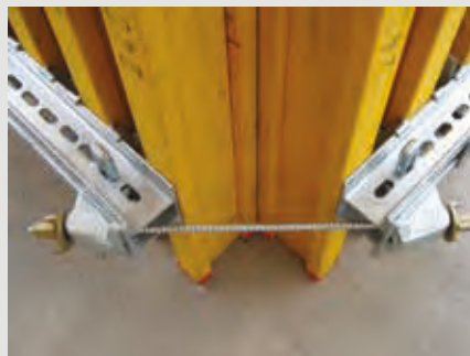
The strong wedge design provides necessary tension through the slotted waler connectors for leak-proof joints, while simultaneously aligning the panels.
